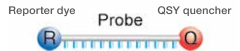
Figure 1. QSY probe. The newly developed QSY quencher can be used in multiplex qPCR with FAM™, VIC™, ABY™, and JUN™ reporter dyes. The QSY quencher is nonfluorescent, leading to less background and improved quenching efficiency.
