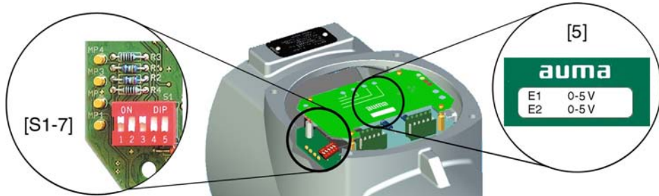
Figure 37: Version with additional switch on the positioner board
