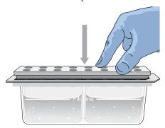
Note: The CBC is filled significantly above Fill Line to account for evaporation. Replace the CBC when the fluid level drops below the Fill Line.
