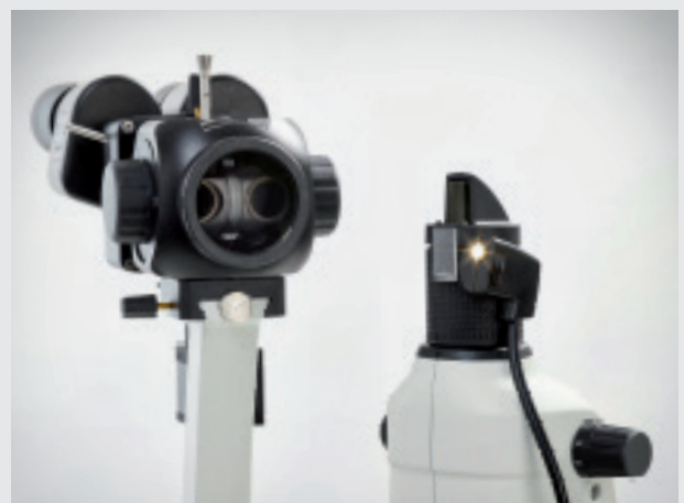
Background illumination system of the SL-IC4 D
