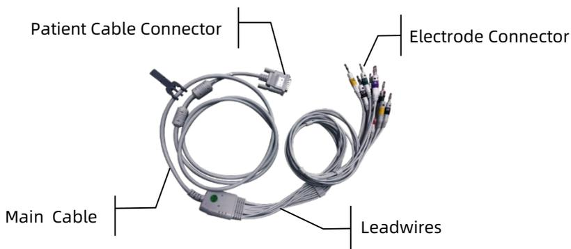
The patient cable consists of a patient cable connector, main cable, leadwires (4 limb lead wires and 6 chest lead wires) and electrode connectors:
