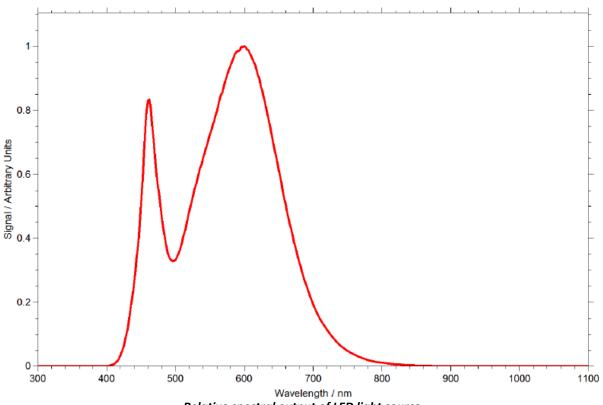
Relative spectral output of LED light source
