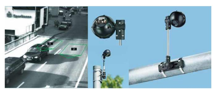
With the Sivicam, detection zones can be precisely demarcated and supervised
