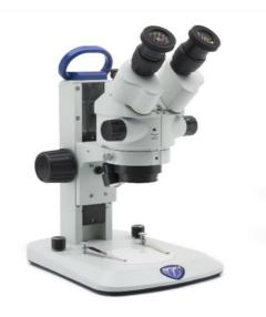
Trinocular stereozoom microscope, 7x...45x
