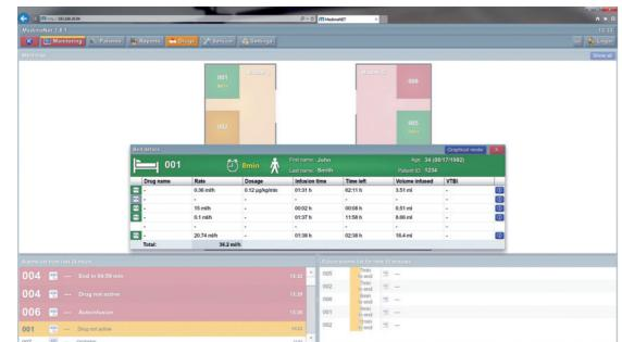
Centralized alarm system indicates pumps currently in active operation requiring intervention. Remaining infusion time list indicates incoming events.
