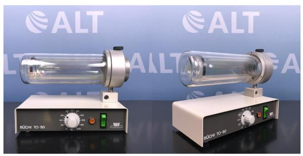
The **Buchi TO-50 Analog Drying Glass Oven** effectively removes moisture from products. The adjustable temperature and time control gives you the option to keep the sample in motion.
