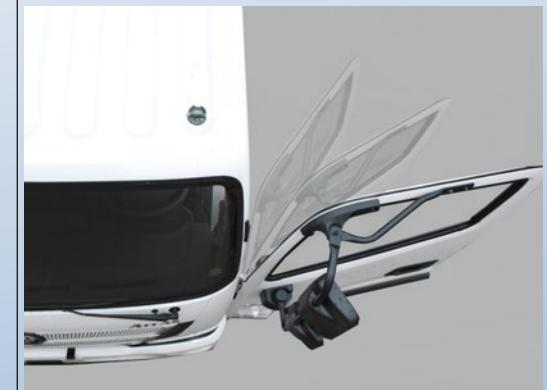
Reinforced Side Doors that Can Be Gradually Opened By 90°
