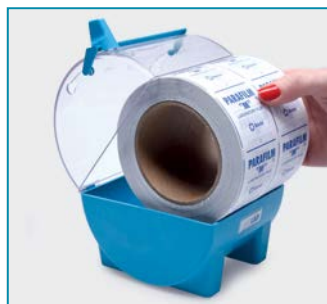
Place the parafilm and move the mechanism back to original position.
