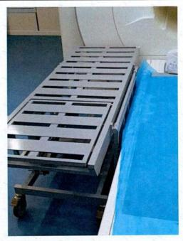
The transfer bed is completely exposed to the 3.0T strong magnetic environment, with the leg part of the transfer bed facing the MR machine (bore side), and the side of the transfer bed is 2~5cm away from the side surface of the examination bed.
