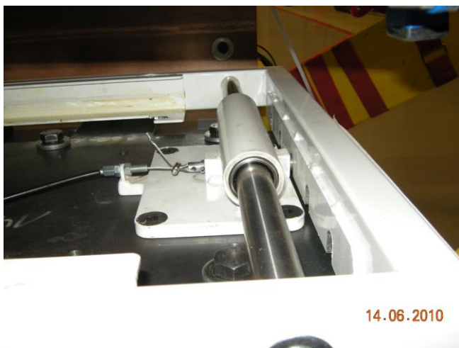
Detail; Floor fixation brackets (foot end side)
