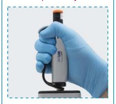
Ejection is simply done applying light pressure to the levered ejector arm.
