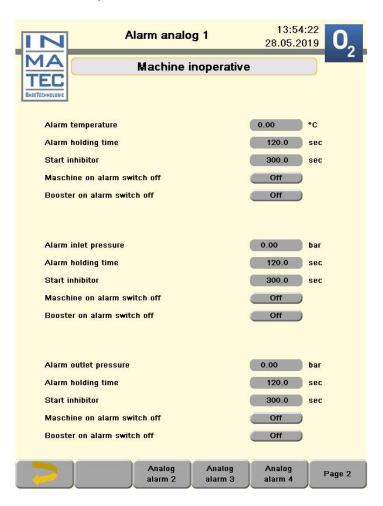
Fig. 11: Alarms control menu: Alarm outlet pressure
