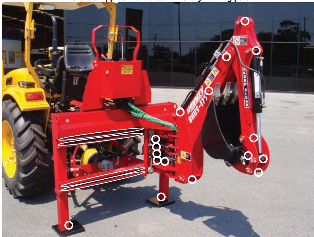
Sliding bars for frame carrier require greasing Total of 19 grease nipples on BHUF & BHUS series Grease nipples are located on every moving part
