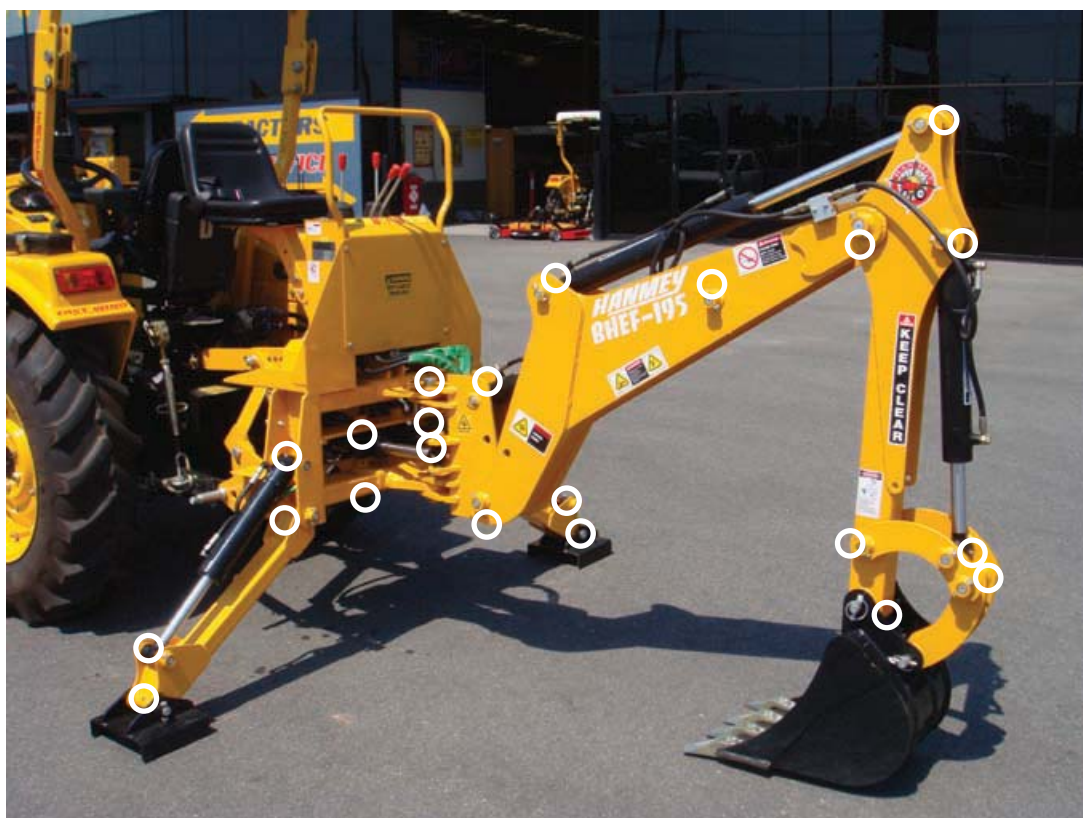
Total of 27 grease nipples on BHEF & BHUF series Grease nipples are located on every moving part
