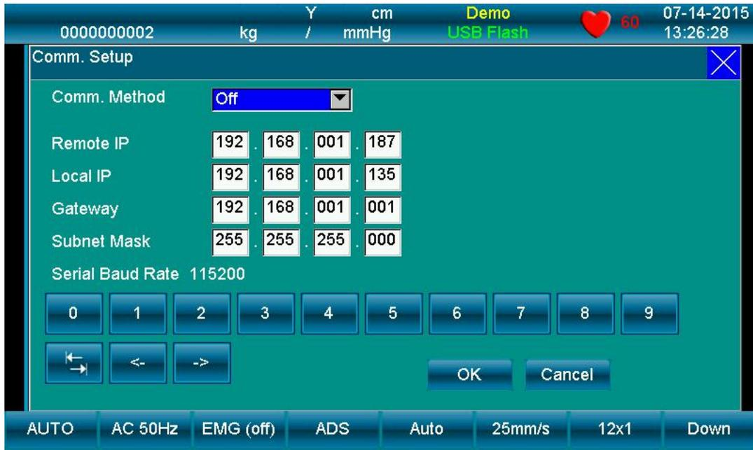
Figure 5-14 Communication Setting Interface
