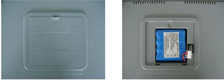
Figure 8-1 Battery Installation
