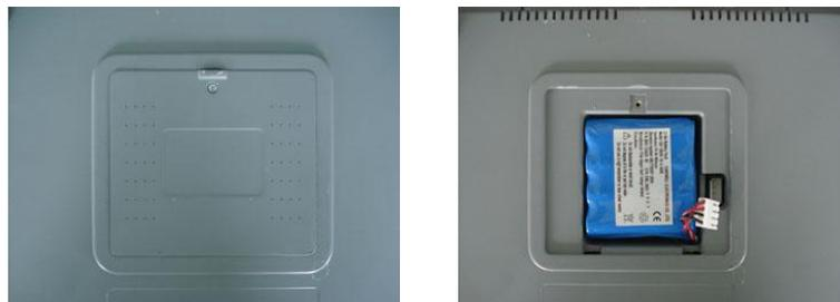
Figure 5-21 Battery installation
