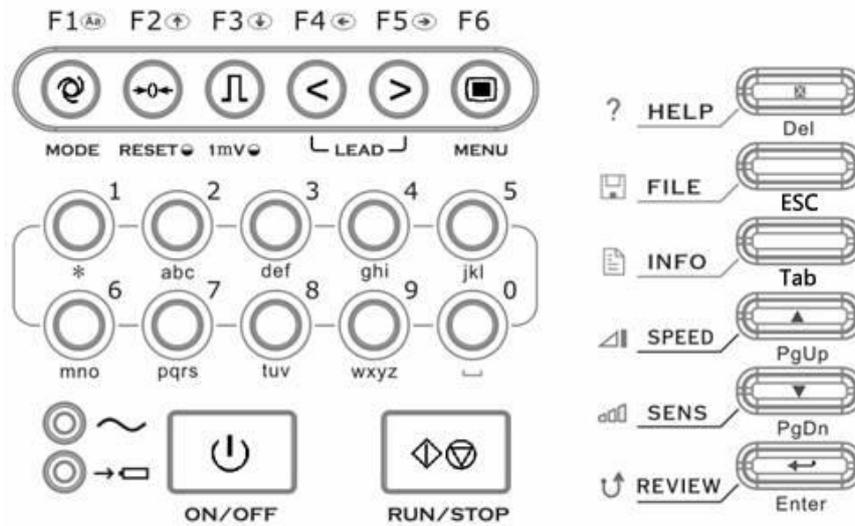
Figure 3-3 Control Panel of ECG-1112M
