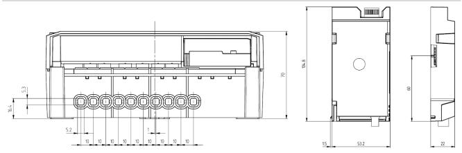
D000063744 en d – E570 Series 2 2G/4G transformer connected 3-phase electricity meter – ZMY/ZFY405CW1, ZMY/ZFY410CW1 – Technical data © Landis+Gyr
