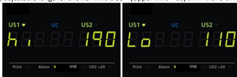
Fig. 3.1 Alarm Upper /Lower Limit
