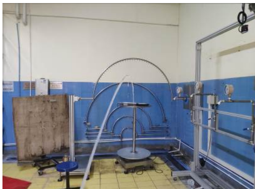
Photo 4 -- During the test of IPX5
