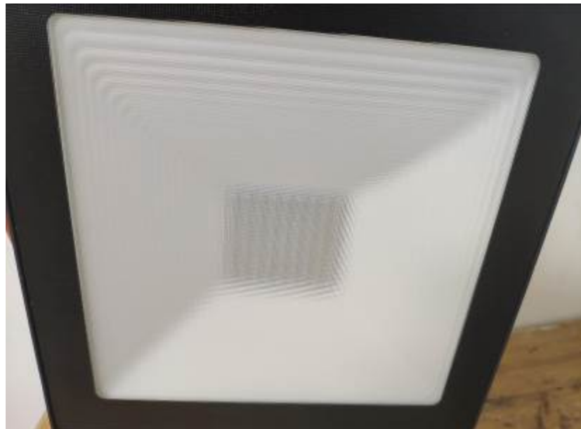
Photo 11 -- After the test of IK08
