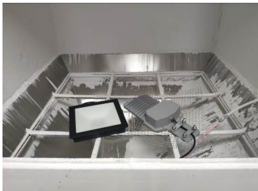
Photo 3 -- During the test of IP6X
