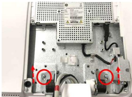
Figure 8-96 Half unscrewing points
