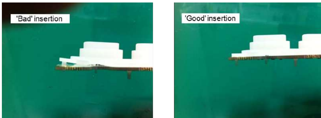
Figure 8-135 Installation of PWA
