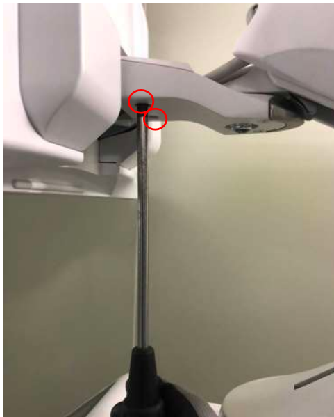
Figure 8-98 unscrewing 2 screws and separating the Pan Arm Down Cover
