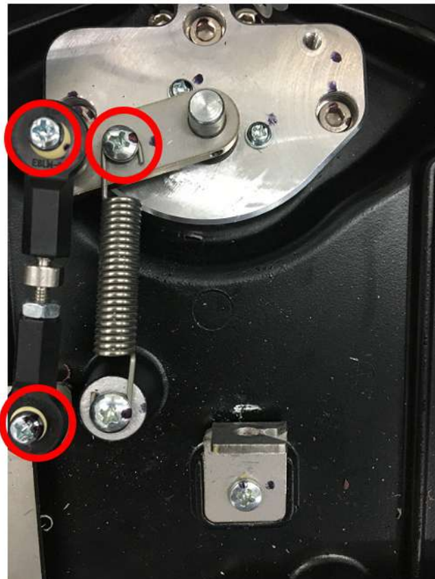
Figure 8-346 Unscrewing 3 screws and removing Turn Buckle Set and Spring
