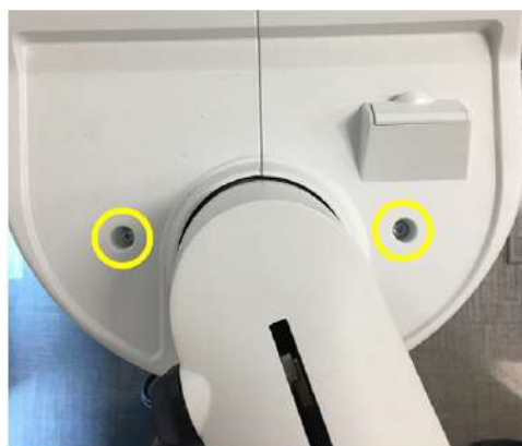
Figure 8-140 Unscrewing 2 screws on OPIO Top Covers
