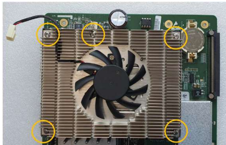
Figure 8-210 Unscrewing five male type screws
