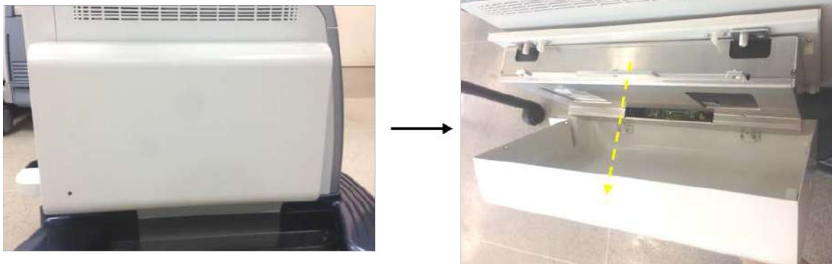
Figure 8-334 Disassembling BATTERY PACK COVER BRKT
