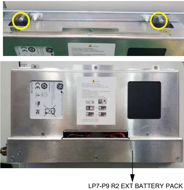
Figure 8-338 Pulling out LP7-P9 R2 EXT BATTERY PACK from BATTERY PACK FRAME BRKT
