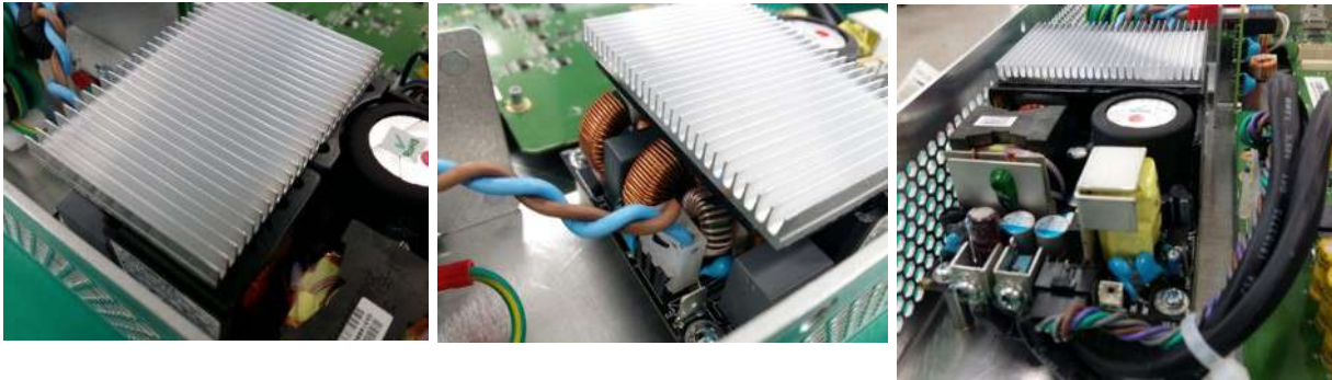
Figure 8-370 Checking the Internal harness
