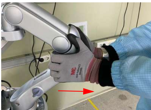
Figure 8-83 Removing 2nd Axis Cover
