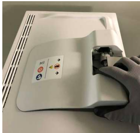
Figure 8-87 Removing the monitor cable cover
