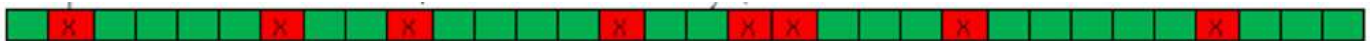
Figure 7-29 Example: 6 of 32 elements are defect with a gap of 2 good elements between (defect elements marked by X)
