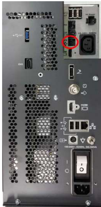
Figure 8-281 Speaker cable connector position
