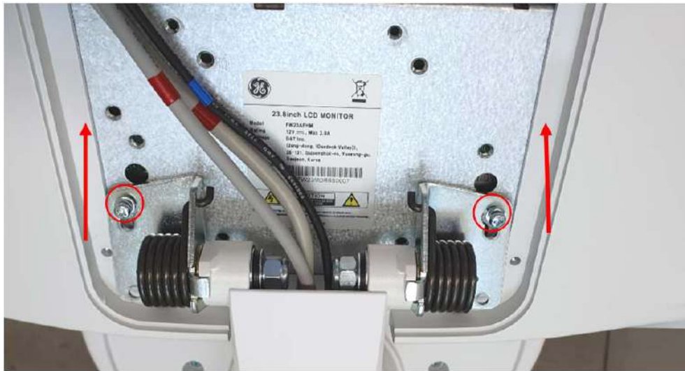
Figure 8-91 Pushing the monitor to remove the monitor
