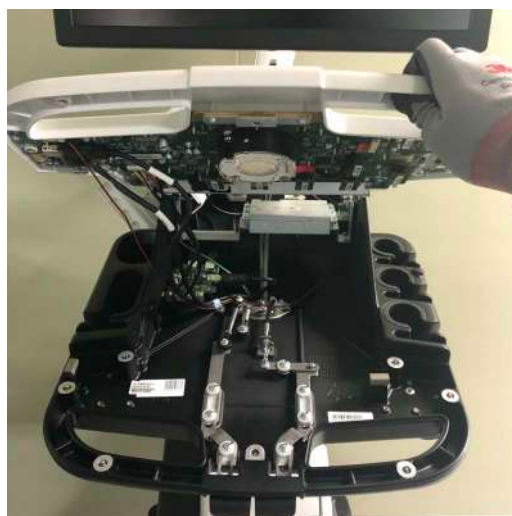
Figure 8-142 Lifting OPIO Assy up
