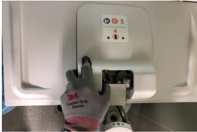
Figure 8-92 Removing the monitor cable cover
