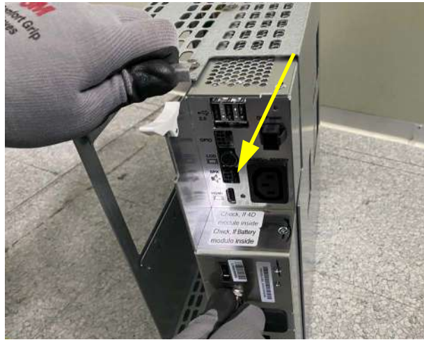
Figure 8-323 Drawing IO BOX from NEST FRAME
