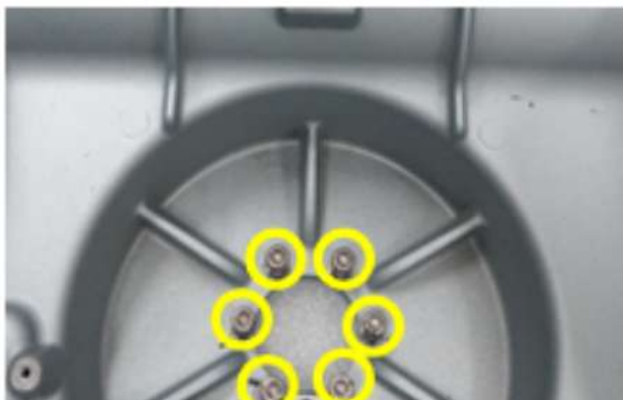
Figure 8-348 Unscrewing 6 screws and detaching OPIO Base
