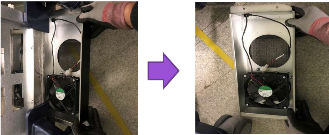
Figure 8-221 Removal of bottom fan Assy
