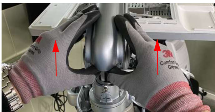
Figure 8-84 Removing 2nd Arm Cover
