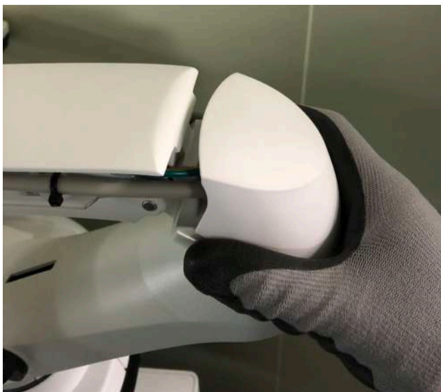
Figure 8-100 Detaching the Joint Cover
