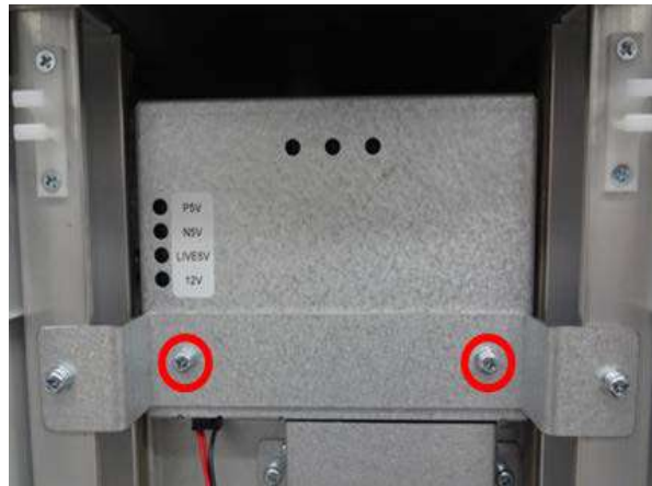
Figure 8-163 Front side screw points
