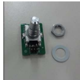
Figure 8-150 unfastening nut and detaching the encoder
