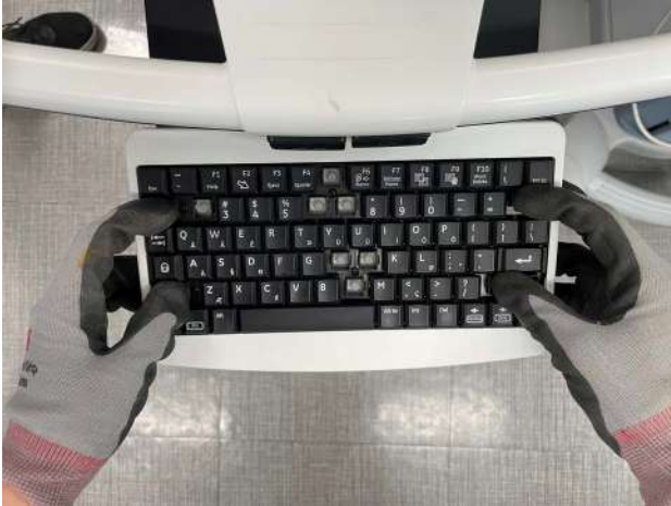
Figure 8-156 Detaching key caps.
