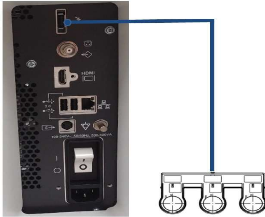
Figure 3-9 Connection Scheme - Footswitch
