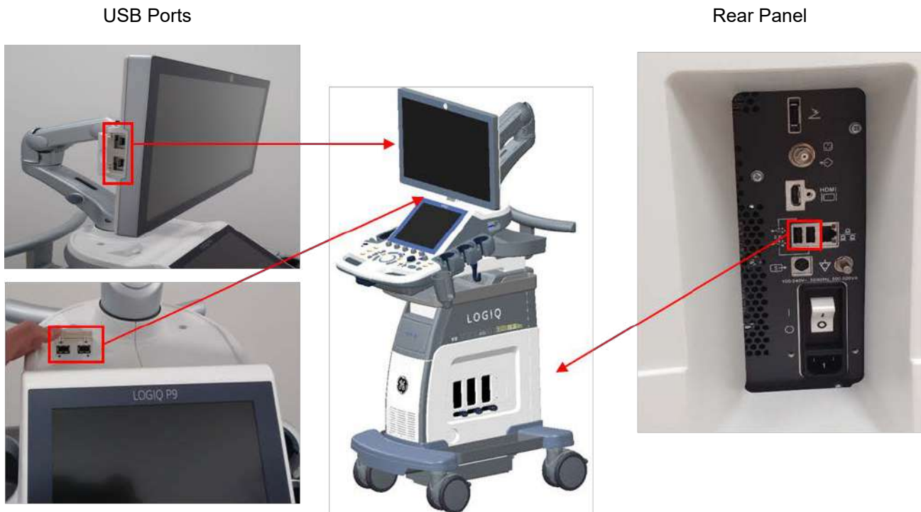
Figure 5-8 System Ports (R1, R2, R2.5 and R3)
