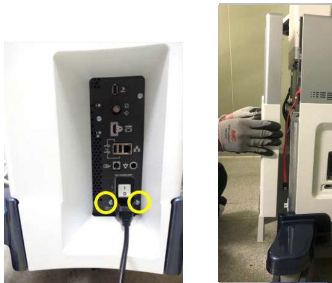
Figure 8-310 Removing POWER CORD FIX BRKT, POWER CORD and REAR COVER
