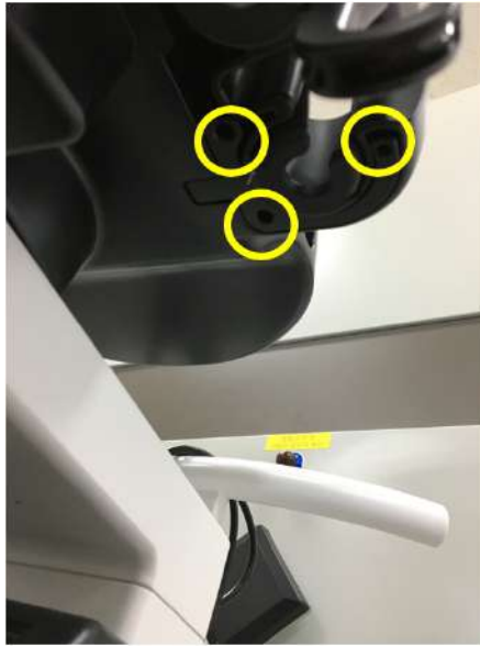
Figure 8-358 Unscrewing 3 screws and detaching the probe light assy
