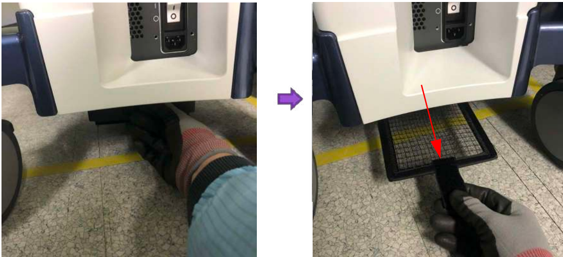
Figure 8-289 Removal of bottom fan filter
