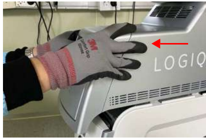
Figure 8-69 Removal of Cabinet
