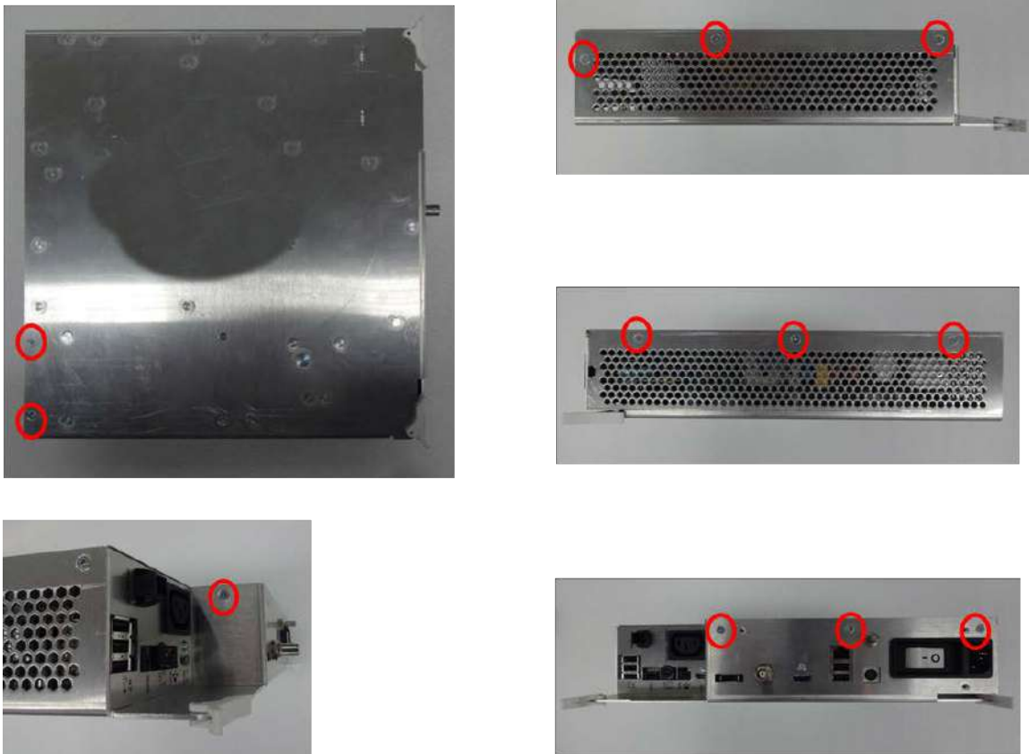
Figure 8-249 Screw points of IO BOX cover
