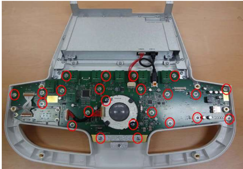
Figure 8-130 Screw points on Main PWA Assy
