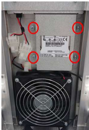
Figure 8-241 Screw points around HDD/SSD Bracket.
