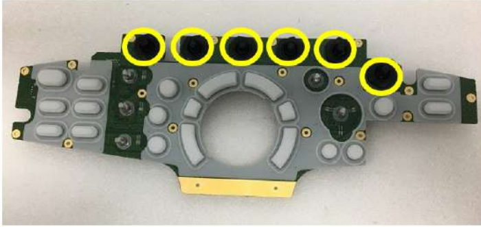
Figure 8-151 Unfastening nut and detaching the Joystick encoder
