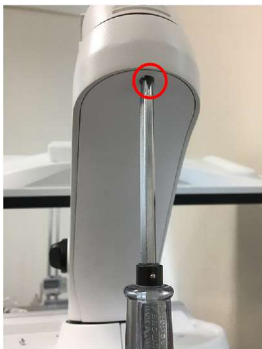
Figure 8-101 Unscrewing 1 screw and detaching the Extension Arm Cover
