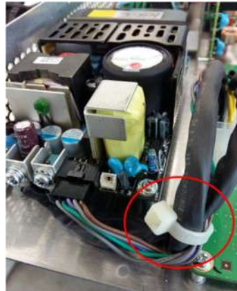
Figure 8-367 Tightening the harness
