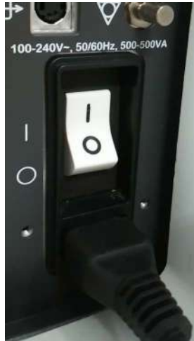
Figure 8-316 Turning on circuit breaker
