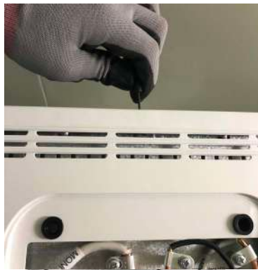
Figure 8-104 Unscrewing 4 screws and separating Monitor Rear Cover
