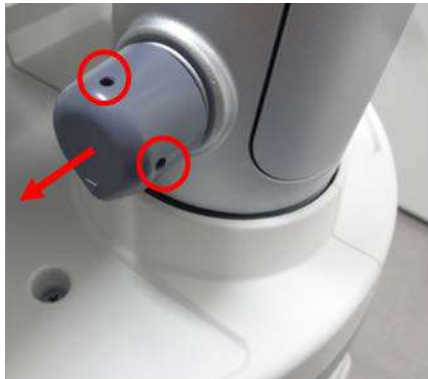
Figure 8-109 Fixed Arm Holder Grip Cover screw points
