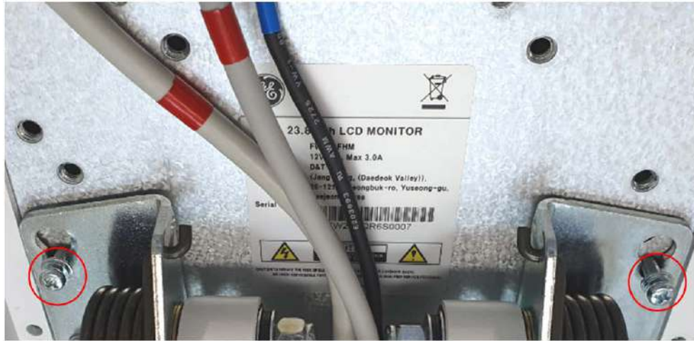
Figure 8-90 Halfway unscrewing points
