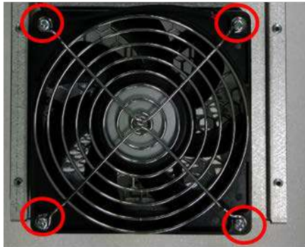
Figure 8-218 Fan screw points and disconnecting fan connector
