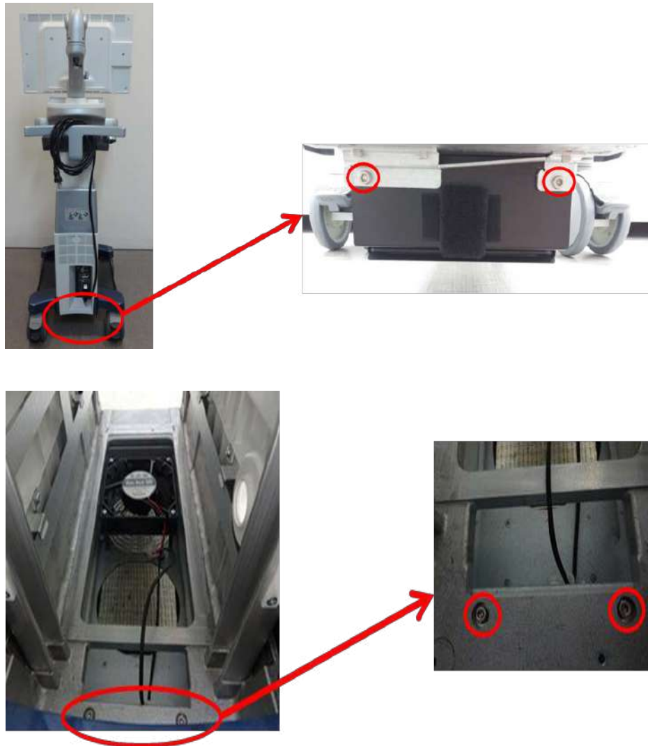
Figure 8-219 Fan screw points of bottom fan assy
