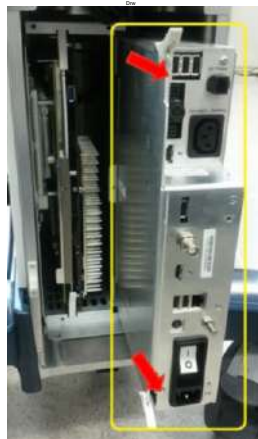
Figure 8-363 Drawing the IO Box from Nest Frame
