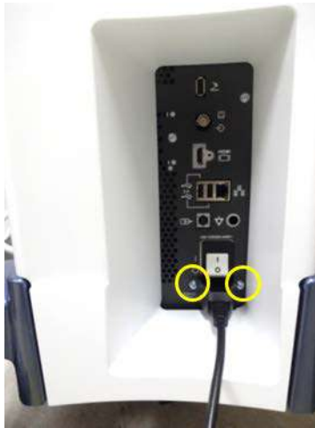
Figure 8-319 Removing POWER CORD FIX BRKT and POWER CORD
