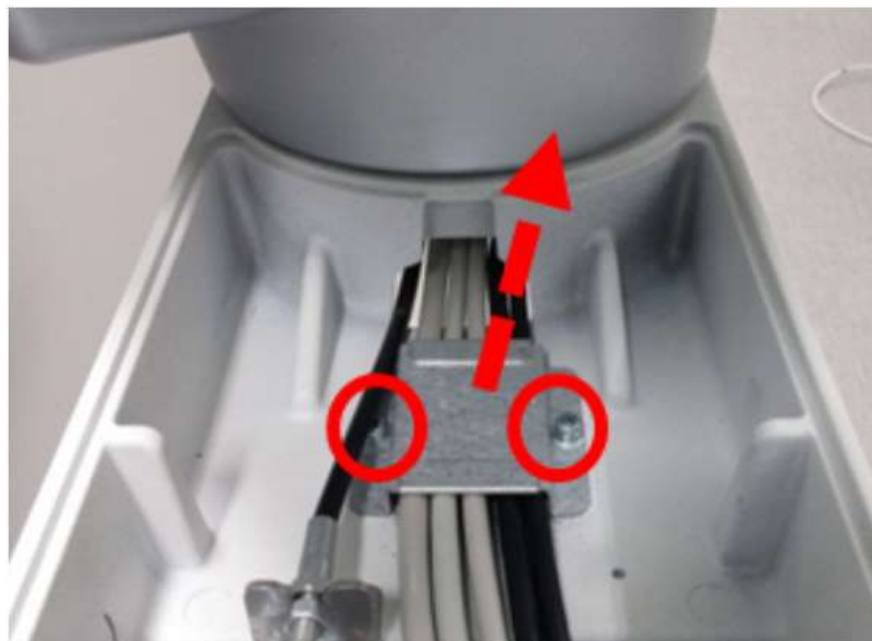
Figure 8-260 Unscrewing 2 screws and removing 2 cables
