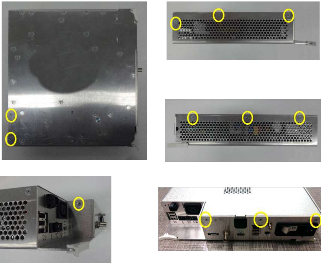
Figure 8-313 Unscrewing 12 screws to remove MIO BOX BRKT
