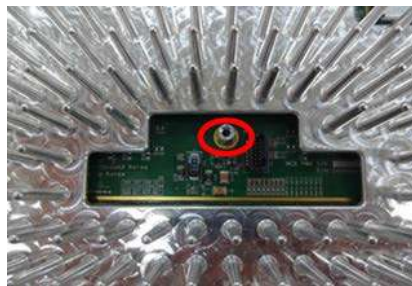
Figure 8-198 Stud position on MCB board.
