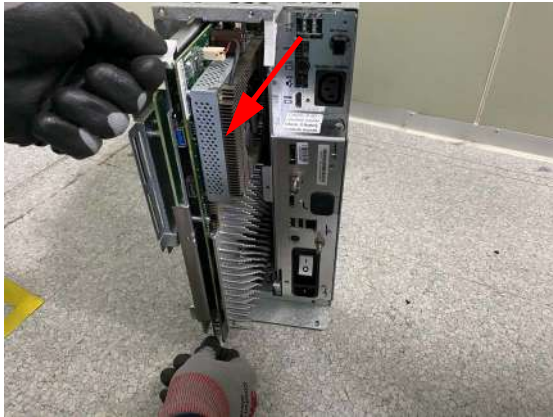
Figure 8-167 Separating Board Assy
