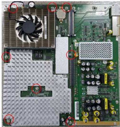
Figure 8-244 Removal of eight screws
