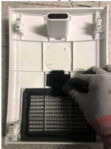
Figure 8-288 Pulling out the front fan filter.
