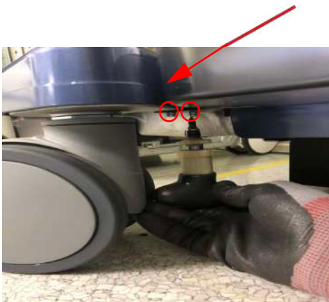
Figure 8-75 SIDE TRAY FIX BRKT screw points
