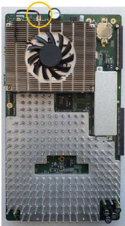
Figure 8-209 Disconnecting fan cable
