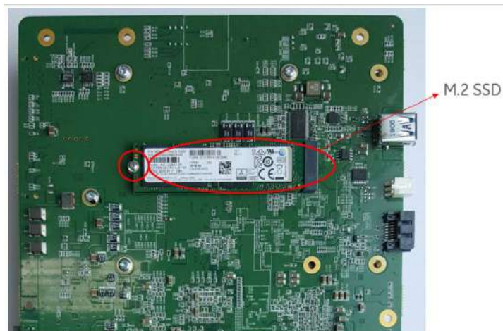
Figure 8-245 Removal of one screw on bottom side of the board
