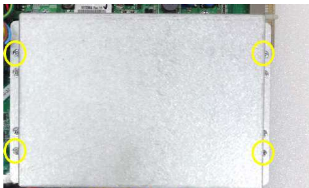
Figure 8-326 Disassembling BATTERY ASSY
