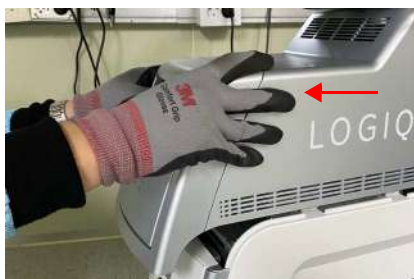
Figure 8-66 Removal of Cabinet
