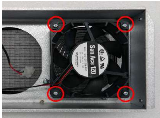
Figure 8-222 Screw points of bottom fan.
