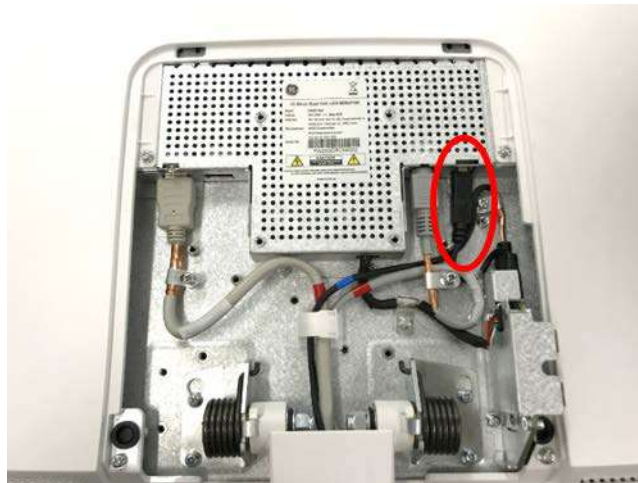
Figure 8-93 Disconnecting USB cable
