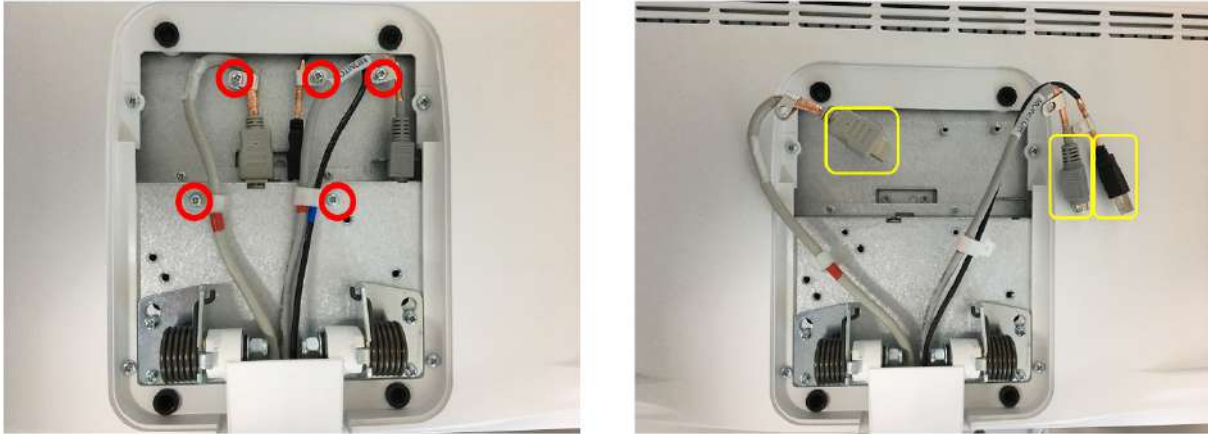
Figure 8-88 Unscrewing 5 screws and disconnecting monitor cables
