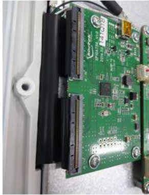
Figure 8-136 Installation of Touch panel connector
