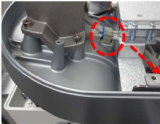
Untying the cable clamp
