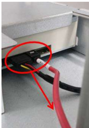
Figure 8-264 Removal of DVD cables from the DVD
