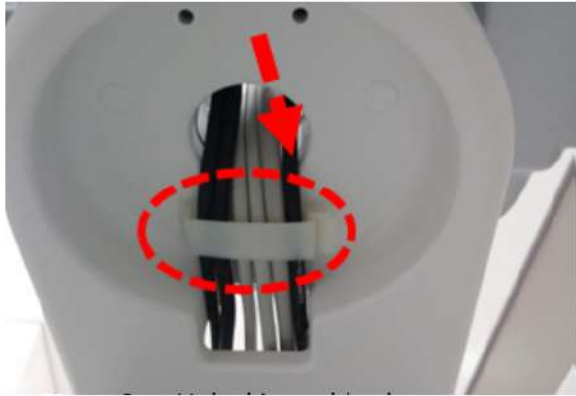
Unlocking cable clamp
