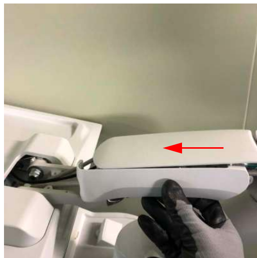
Figure 8-99 unscrewing 2 screws and detaching the Lift Arm Cover L, R
