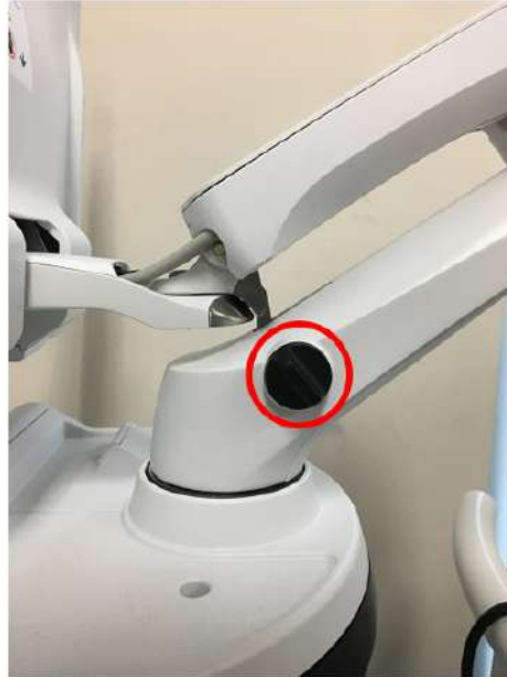
Figure 8-86 Locking the Monitor Arm
