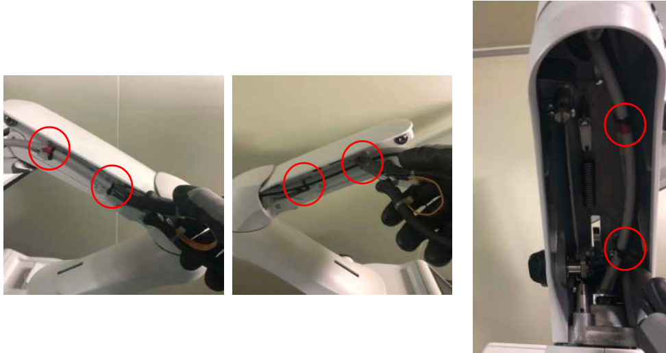
Figure 8-255 Cutting 6 cable ties
