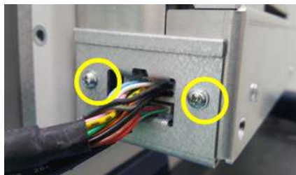
Figure 8-301 Unscrewing 2 screws to remove CONNECTOR BRKT
