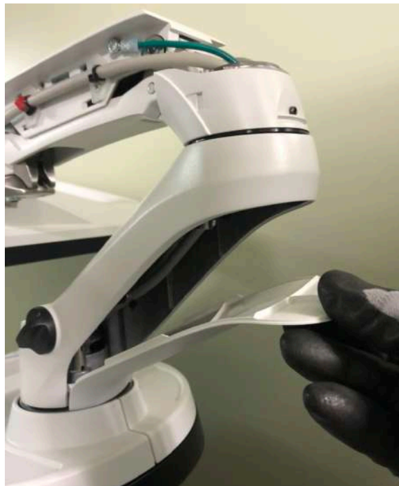
Figure 8-101 Unscrewing 1 screw and detaching the Extension Arm Cover
