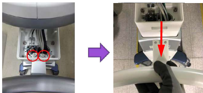
Figure 8-224 Hex screw points of Rear Handle
