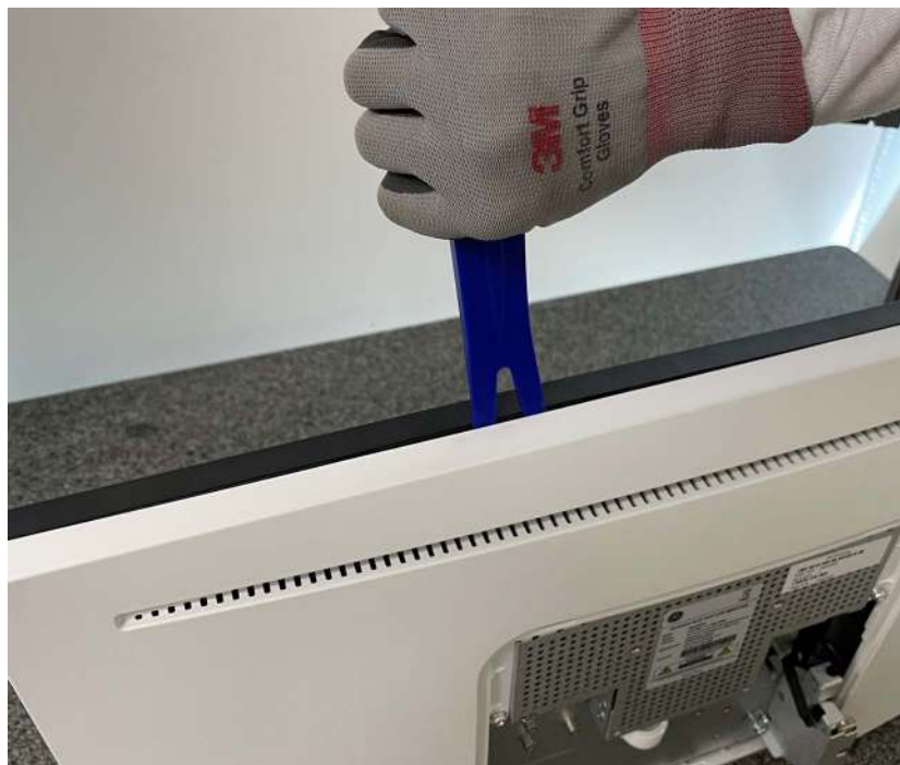
Figure 8-106 Unscrewing 4 screws and separating Monitor Rear Cover
