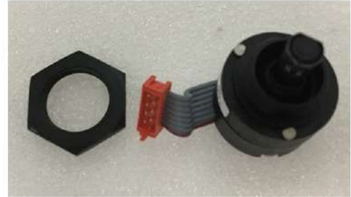
Figure 8-151 Unfastening nut and detaching the Joystick encoder
