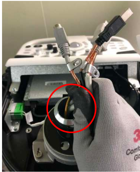
Figure 8-258 Extracting 3 monitor cables
