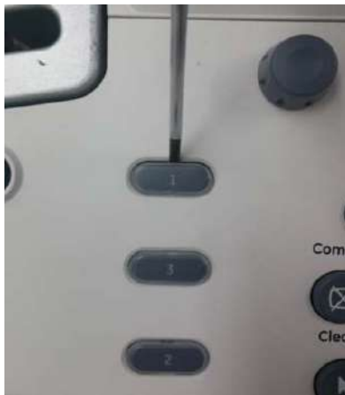
Figure 8-152 Push against the circle cap and lift it
