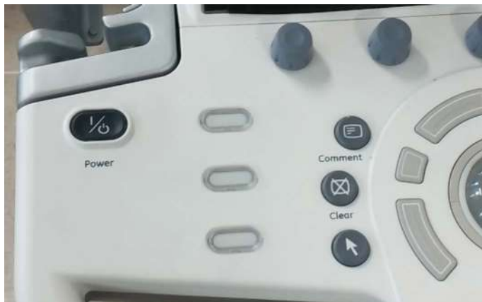
Figure 8-308 Booting-up using power button
