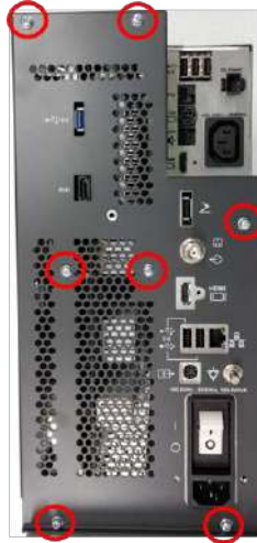
Figure 8-166 Screw points on Nest Box
