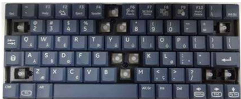
Figure 8-155 Loosen the 6 screws
