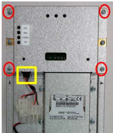
Figure 8-213 Screw points and connector point to remove MBP
