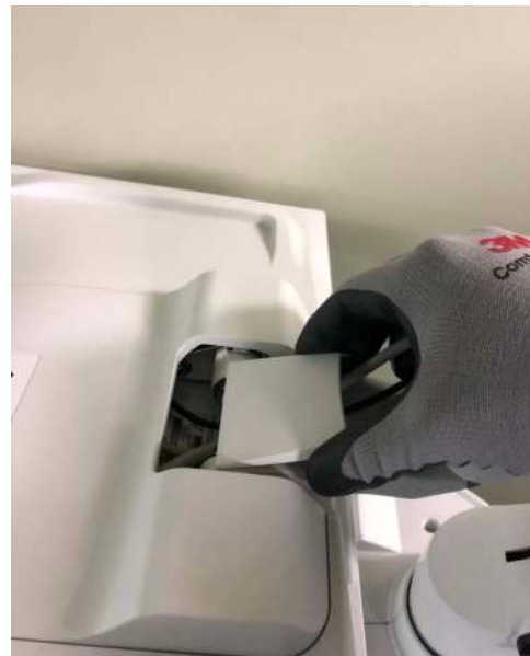
Figure 8-98 unscrewing 2 screws and separating the Pan Arm Down Cover
