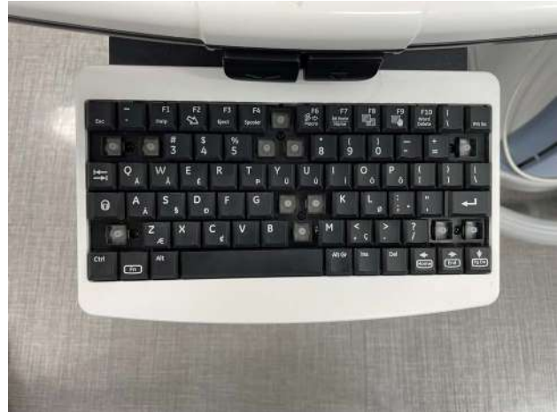
Figure 8-156 Detaching key caps.
