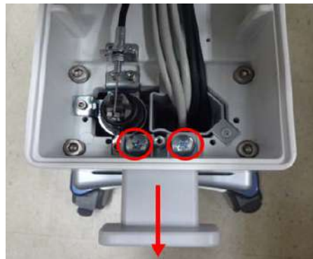
Figure 8-226 screw points of Link Arm Cable Hook
