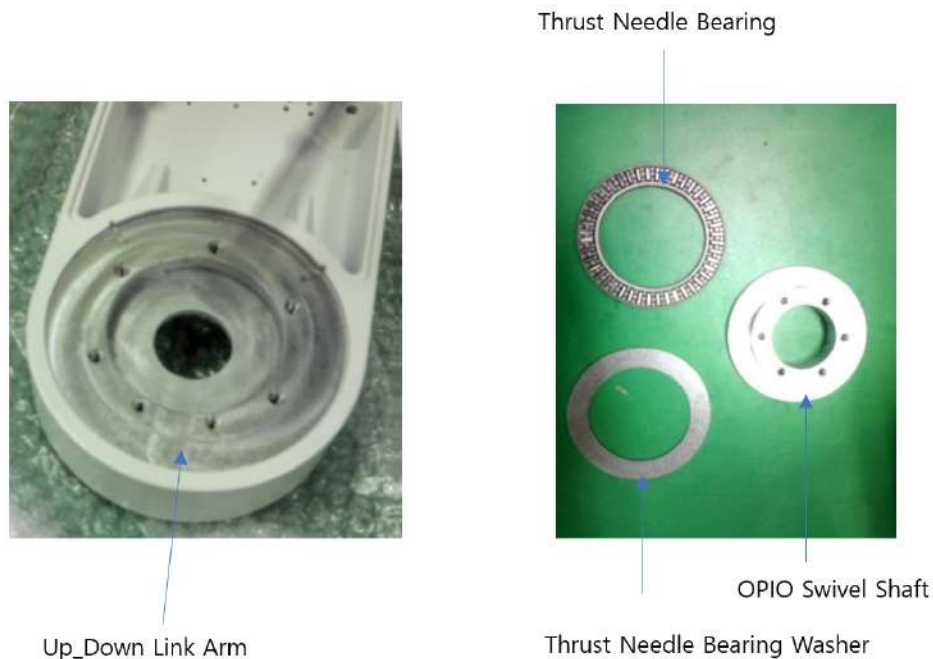
Figure 8-352 Detaching Thrust Needle Bearing Washer, Thrust Needle Bearing, OPIO Swivel Shaft
