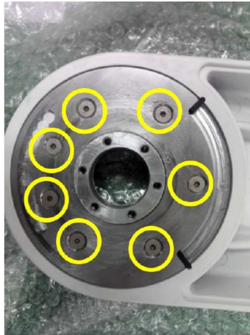
Figure 8-351 Unscrewing 7 screws and removing Rotation Plate
