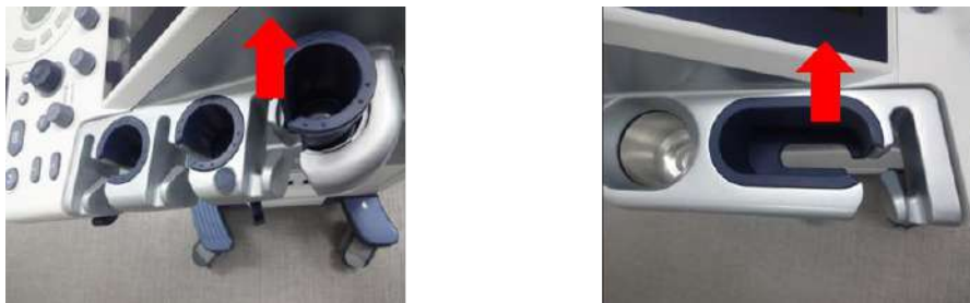
Figure 8-272 Removal of Probe Holder
