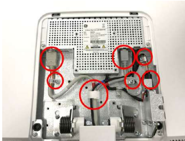
Figure 8-94 Unscrewing 3 screws and disconnecting monitor cables
