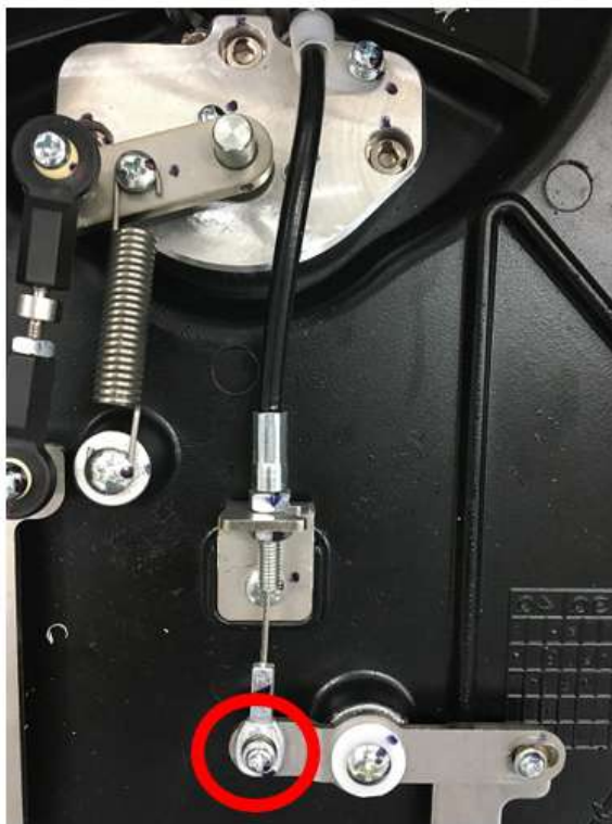
Figure 8-343 Unscrewing 1 screw and disassemble the cable wire
