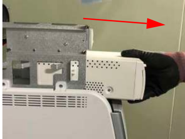
Figure 8-279 Pulling out the BW printer
