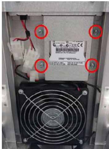
Figure 8-202 Screw points around HDD Bracket.
