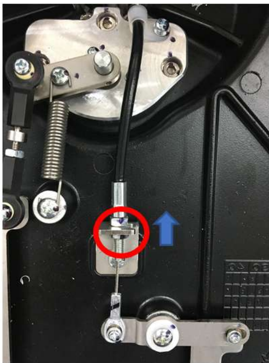
Figure 8-344 Unscrewing nut and disassemble the cable wire
