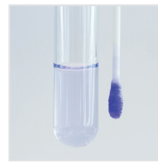
Figure 6. Traditional fiber swabs: the sample stays entrapped in the fiber wad.
