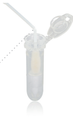
Figure 9. Prescored breaking point.
