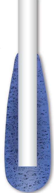
Figure 6. Traditional fiber swabs: the sample stays entrapped in the fiber wad.
