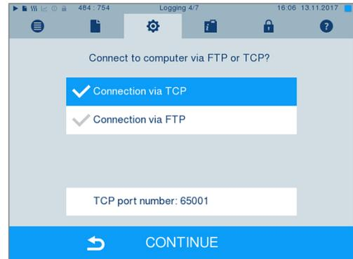
2. Press on the lower pushbutton to change the pre-set TCP port. The display switches to the settings window.
