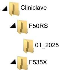
The steam sterilizer checks the memory medium after every type of log output (Immediate output after completed program run or transfer of several logs at once). If a directory does not exist, it automatically creates a directory for the device and the month. If the logs are subject to multiple outputting on the identical memory medium, the device directory will create a "Duplicate" directory.
