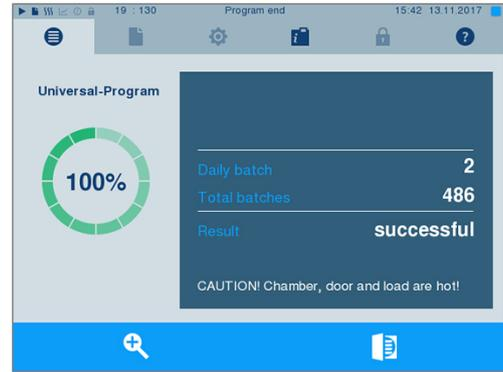
If automatic logging after program end is activated (= Immediate output) in the **Settings > Logging** menu, the log of the completed program will be outputted to the activated output medium after opening the door.
