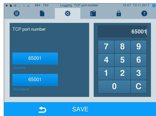
3. Delete the most up-to-date TCP port using key C; enter another TCP port.
