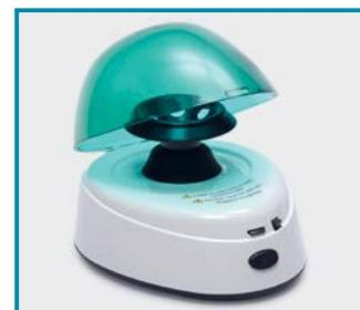
**Easy to stop:** Open the lid, the electrical brake immediately stops the rotor.
