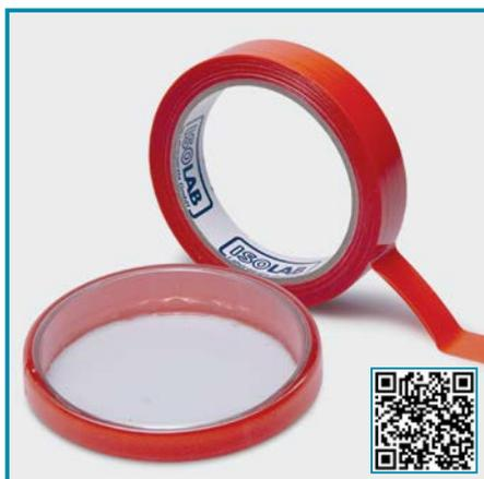
➤ Perfect tool to protect petri dish interior contents. Stretches and widens up 50% of original length.
