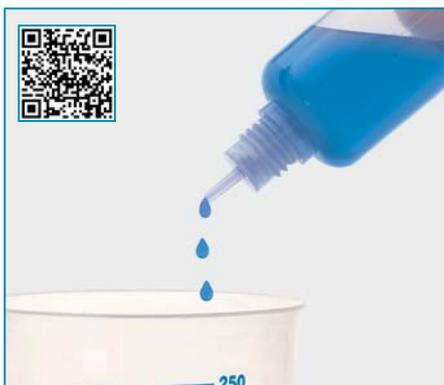
➤ Manufactured from transparent polyethylene with a dropping cap. Cap can be easily dismantled for cleaning.
