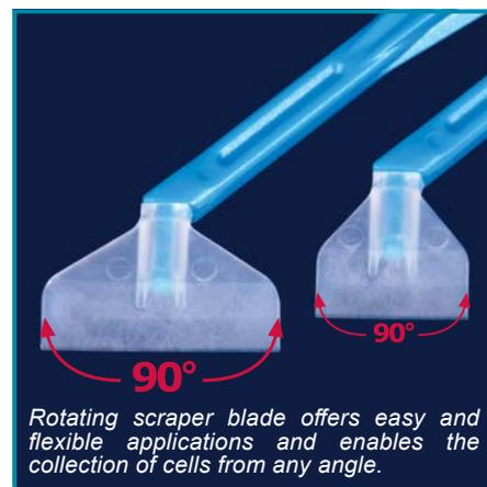
Rotating scraper blade offers easy and flexible applications and enables the collection of cells from any angle.
