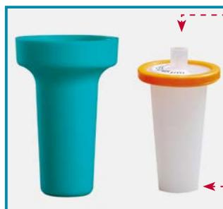
Replaceable hydrophobic 0,45 µm PTFE filter secures cross contamination.
