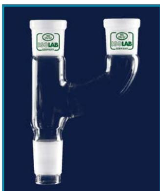
► Manufactured from heat resistant, durable borosilicate glass featured with a parallel socket.
