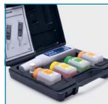
Meters are supplied in a sturdy carry case complete with hand held stripe, pH buffer solutions, cleaning solution, instruction manual and other standard accessories.
