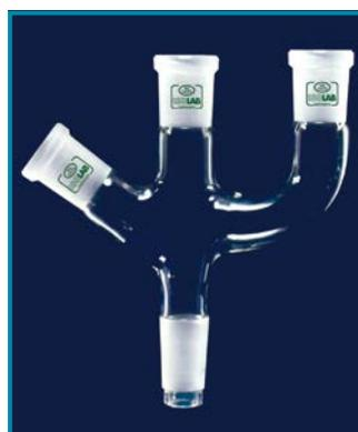
► Manufactured from heat resistant, durable borosilicate glass featured with one parallel and one angled socket.
