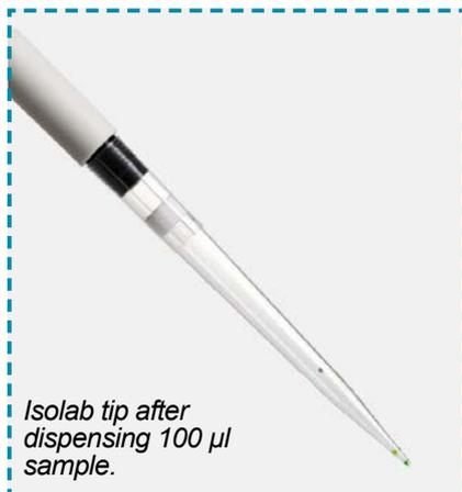
Isolab tip after dispensing 100 µl sample.
