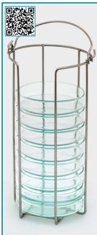
➤ Manufactured from high quality, chemical and corrosion resistant AISI 304 grade stainless steel.
