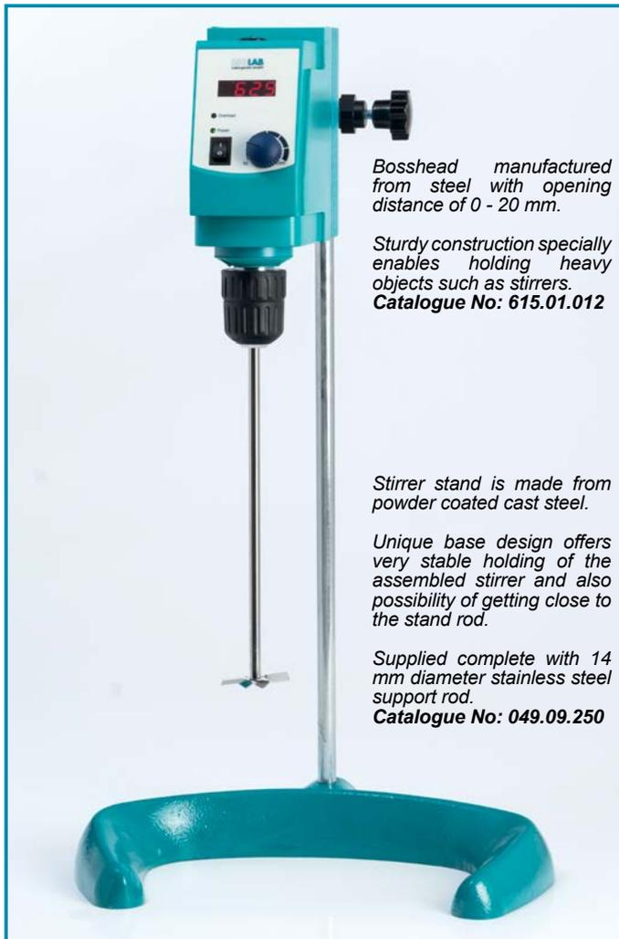
Bosshead manufactured from steel with opening distance of 0 - 20 mm.
