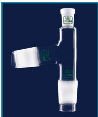
▶ Manufactured from heat resistant, durable borosilicate glass according to DIN 12594 standard featured with a 75° downwards angled cone.
