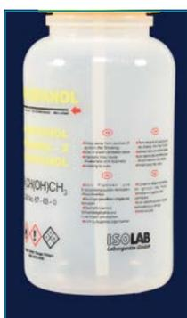
Warning words as "flammable", to identify the the hazardous liquids, "how-to-use" instructions in four languages are printed on the body.
