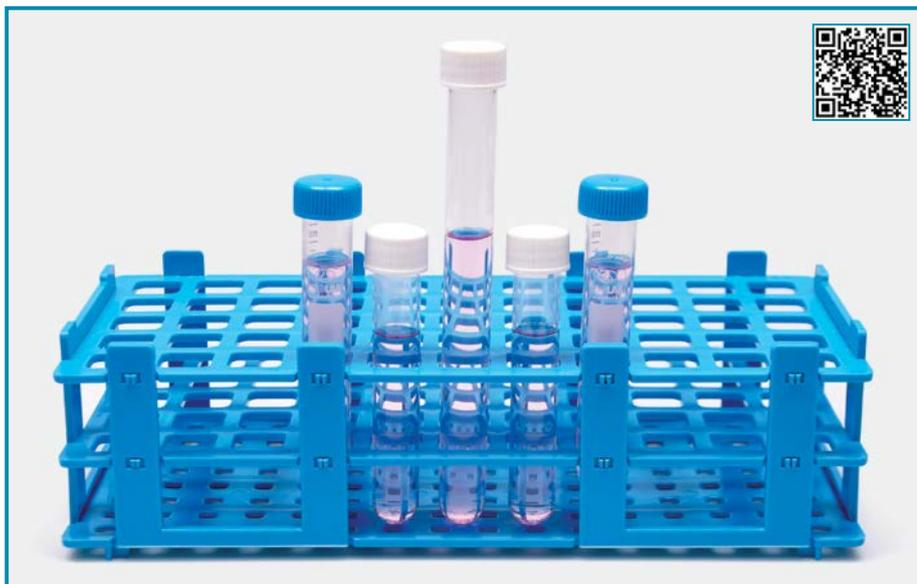
➤ Manufactured from modified polypropylene which enables the racks to be used in water baths without floating.
