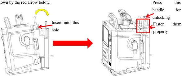
4) Use four M4 screws to fix the bracket with the host through the hole in the red circle shown in the figure below from the bottom of the bracket.
