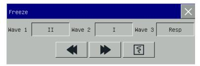
In the [Freeze] window, use the rotary knob to select the forward or backward key and then rotate the knob to move the frozen waveform leftward or rightward. A down arrow is shown on the right side above the top waveform, with a time scale displayed to the left of the arrow. The freeze time is marked as [0s 1]. With the leftward movement of the waveform, the time scale will change to [-1s 1], [-2s 1], [-3s 1]... in sequence, indicating that how many seconds the waveform has been frozen.
