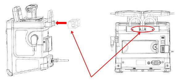
2) Use four M5 screws to fix the bracket on the ambulance through the hole in the red circle shown in the figure below.
