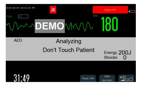
In AED mode, the Defibrillator Monitor will only display one ECG waveform detected by pads and HR value calculated from this displayed waveform. The AED message area at the middle of AED interface will display AED prompt message, contact impedance indicator (settable), shock times and so on.
