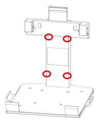
3) Put the monitor on the bracket, and then tilt it to the wall, and fix the monitor to the bracket through the hole shown by the red arrow below.
