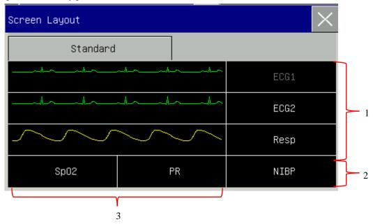
Area 1:Waveform area: You can choose to display the parameters and their waveforms (if one exists). The first row of this area always shows the first ECG waveform and parameter. Waveforms are displayed on the left and parameters on the right. The waveform and its corresponding parameter are shown on the same line.
