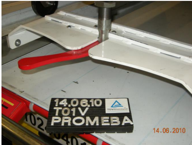
Stretcher fixation (rear lock)
