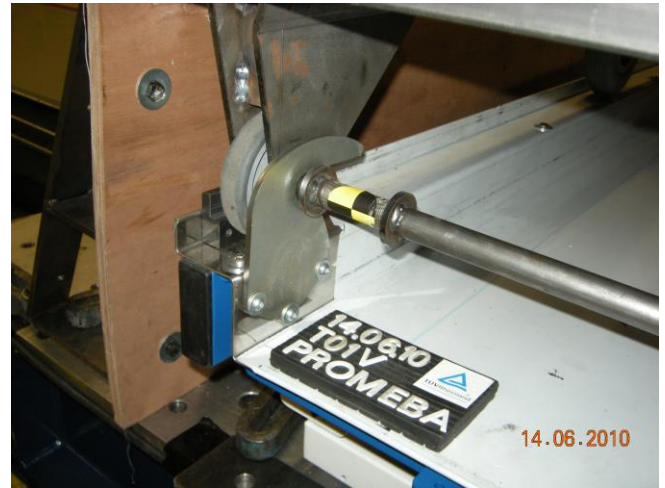
Stretcher fixation (front retention hook)
