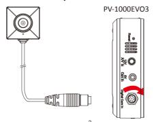
To connect the camera to the DVR, fully plug the camera's connector end into the Digital Cam In port on the DVR, then lock the connector firmly by rotating it to the direction of the red arrow.
