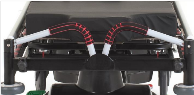
Pushing handles are foldable and removable
