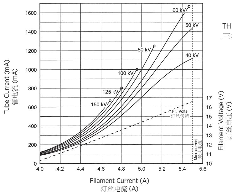
Note: When using these emission curves for trial exposures, refer to the power rating curves shown for maximum kV, tube emission, filament current, exposure time, and target speed.
