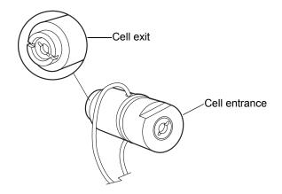
For replacement parts for the TaperSlit flow cell, use the Flow Cell Rebuild Kit.
