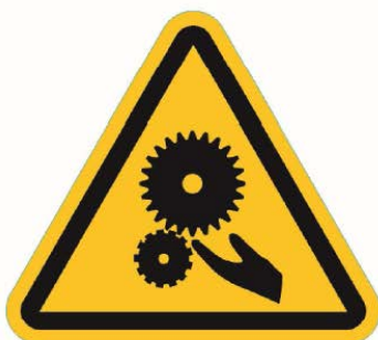
Risk of fingers being crushed
