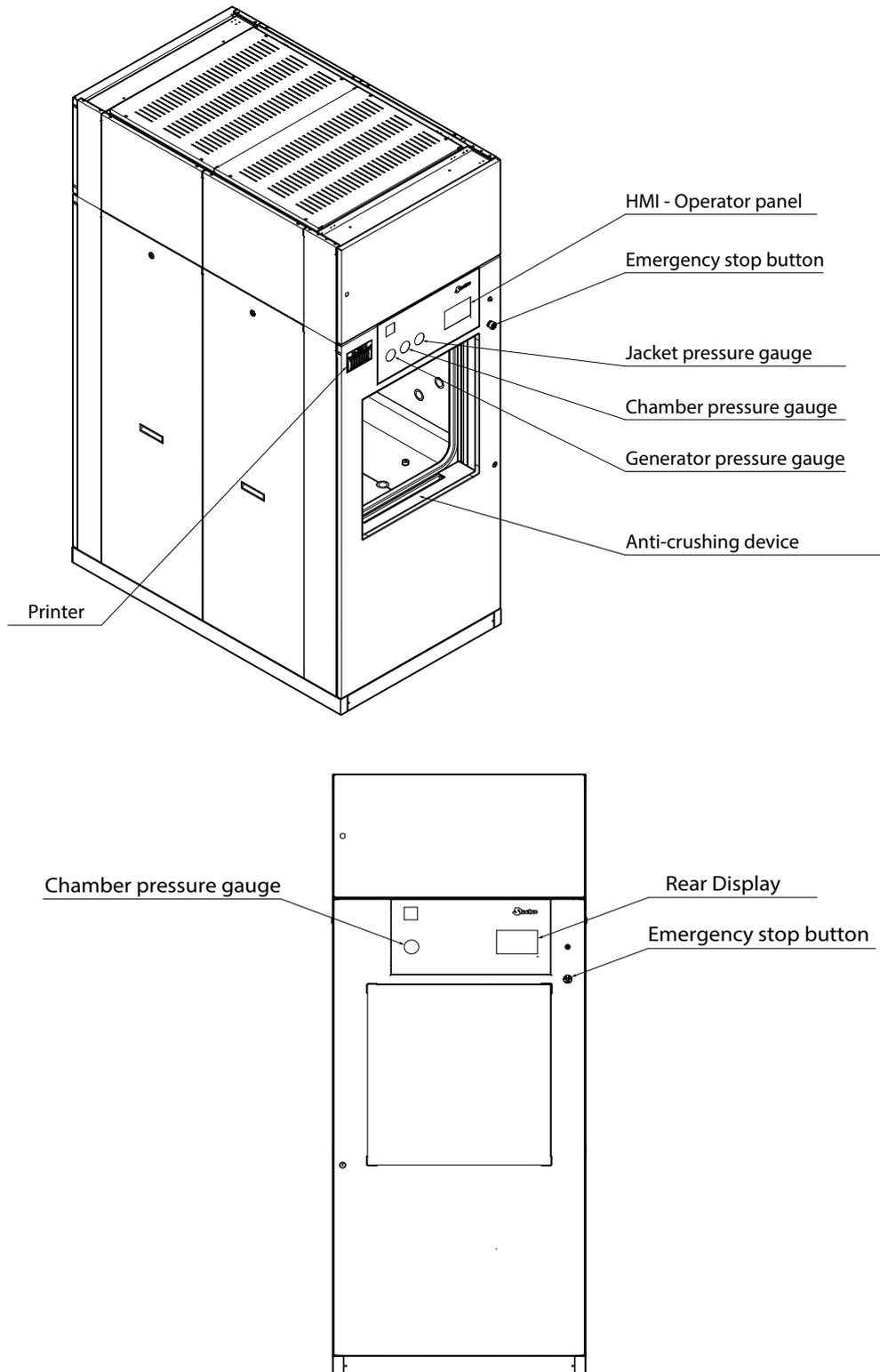
Figure 1 – Identification of front and rear parts
