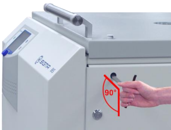
Fig. 48: The emergency lid release key must be inserted horizontally.
