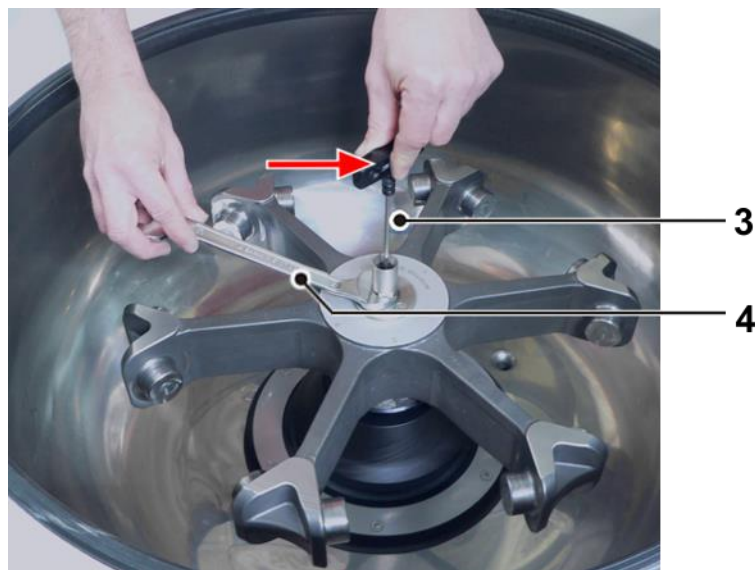
Fig. 20: "Two-finger-principle" for holding the hexagon key
