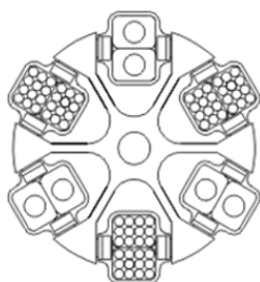
Fig. 22: Permissible and impermissible loading of a swing-out rotor with vessels of various sizes (example illustration)
