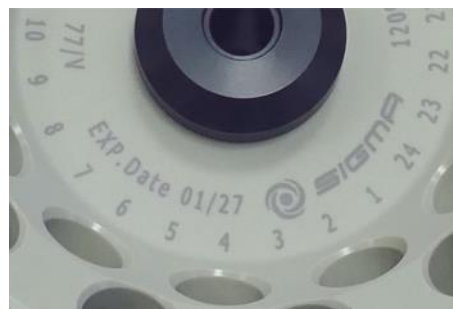
Fig. 8: Different service life – engraving on the bucket/rotor
