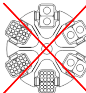
Fig. 22: Permissible and impermissible loading of a swing-out rotor with vessels of various sizes (example illustration)
