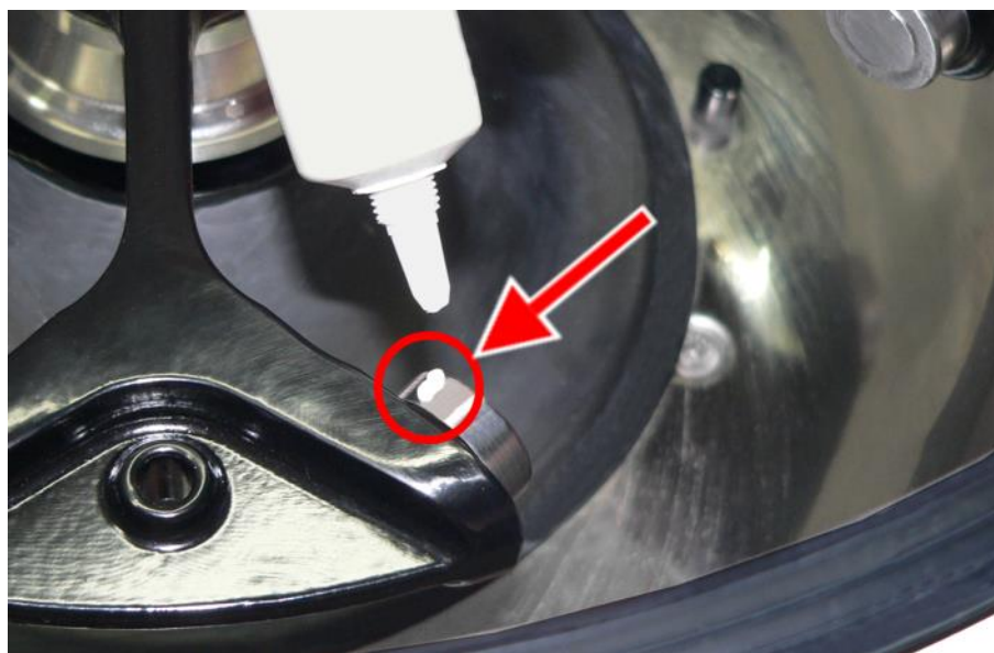
Fig. 49: Sufficient quantity of grease for one bolt
