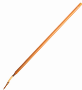
Burette with Rubber Tubing Connection, Glass Bead and Glass Tip
