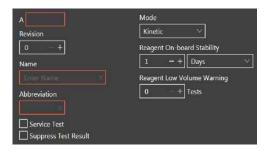
**Test Code** - A three-digit code that represents the test in the analyzer software. The character in front of the code indicates the creator, Predefined tests are identified by a digit or by D (distributor) or S (service). User-defined tests are identified by A (administrator).
