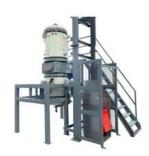
Integrated Autoclave with Shredder (MWI Series) applies to hospitals as well as commercial plants which require higher automation. The system is composed of the autoclave, built-in shredder, supporting platform, automatic bin dumper (except MWI-150), electrical and pneumatic control cabinet, vacuum pump and optional steam generator system.
