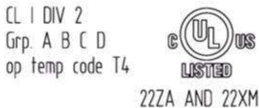
Figure 11: Text Detail – Marking Example for Approved I/O Modules According to NEC 500
