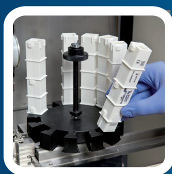
Cuvettes for UriSed 3 PRO (closed system)
