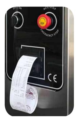
The thermal type printer located in the control unit is supplied with the following values as the cast:
