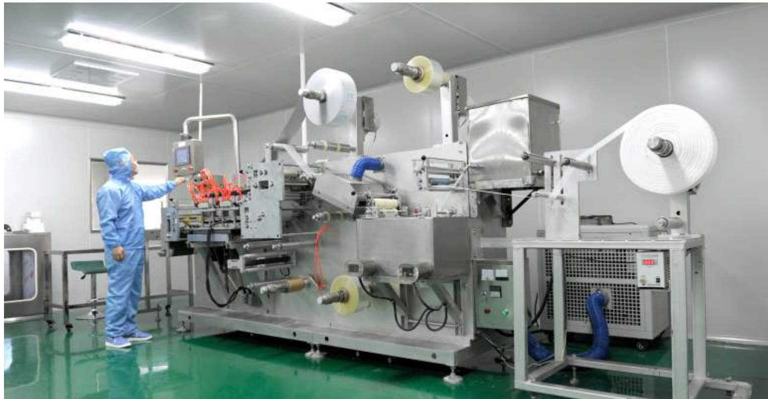
▲ 凡士林纱布片生产线 Production Line for Paraffin Gauze
