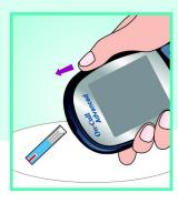
Strip ejector allows easy and smooth strip disposal to avoid contamination
