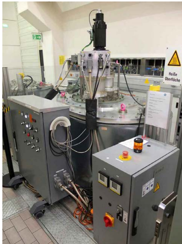
Picture 1: Test setup for the mechanical endurance test and the operation test at 105 °C.
