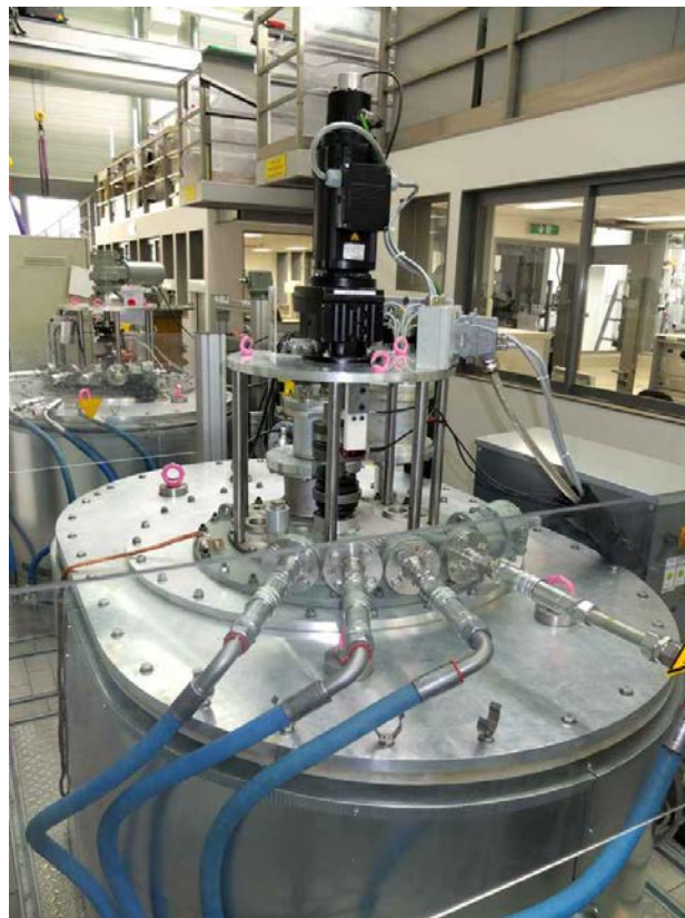
Picture 2: Test setup for the mechanical endurance test and the operation test at 105 °C (heatable test vessel).
