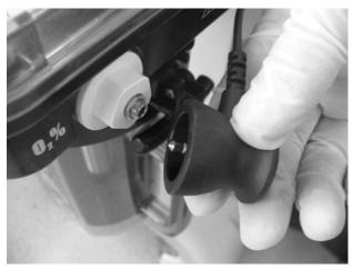
2. Turn the  $O_2$  sensor counterclockwise to take it out.
