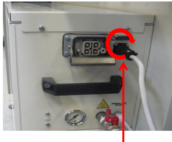
Connect and secure 4Pin AMP round plug and secure its position!
