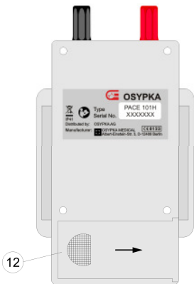
Figure 4: Access to battery compartment
