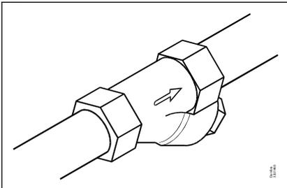
In water applications, exercise the valves at least once every 24 hours, meaning change the state of the valve. The valve exercise will minimize the risk of the valve sticking due to calcium carbonate, zinc or iron oxide build-up.
