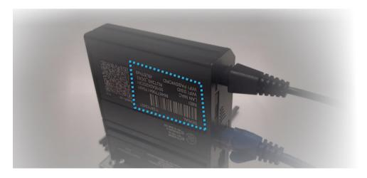
Alternatively, you can connect your computer to TrafficXRoadsvia LAN cable. Access the LTE modem web interface at **192.168.1.1**
