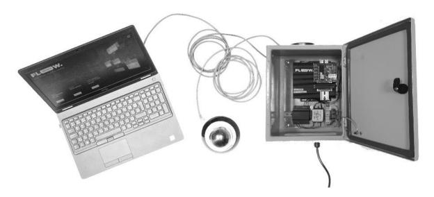
TrafficEmbedded is able to perform in a number of different topologies and setups (as described in the following sections), however, in this phase we will limit ourselves to the simplest configuration - we will connect the computer directly to the internal network of the TrafficEmbedded unit.
