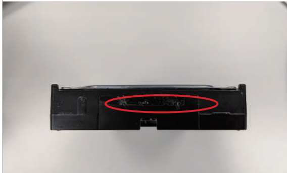
Missing module label
