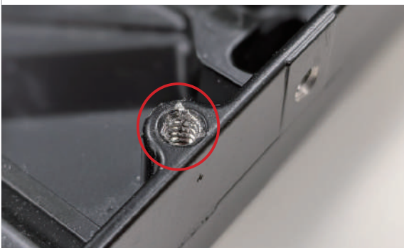
Damaged screw hole
