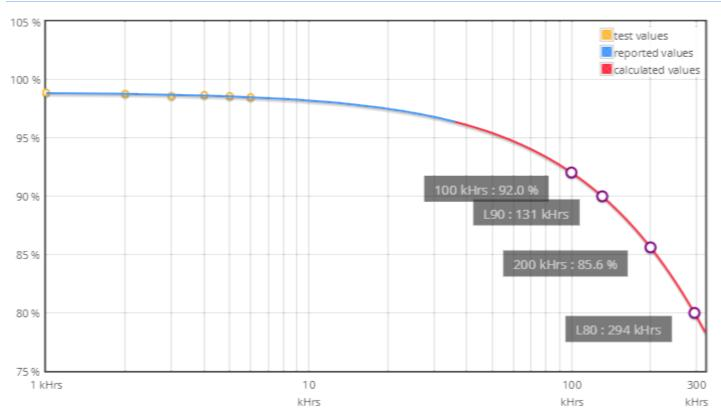
LxB50 results according to LM-80 and TM-21 procedures and norms.
